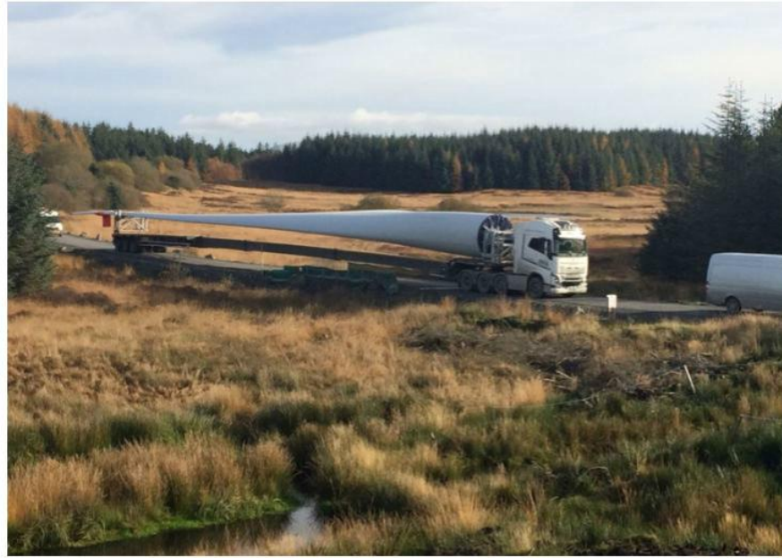
Above: Blade Image shows delivery vehicle with 57 m blade, Harestanes South blades will be up to 75 m in length
